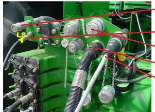
• Case drain, not required in most Exactrix Systems, use with rotary abutment motor. Case drain is normally used with the high speed fan motor. Green Code.
