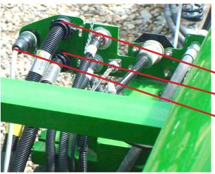
Hydraulic Cylinders Use SCV Remote Connectors Deere 9300 Wheel Tractor shown, 6200 TASC Control, Power Beyond.
