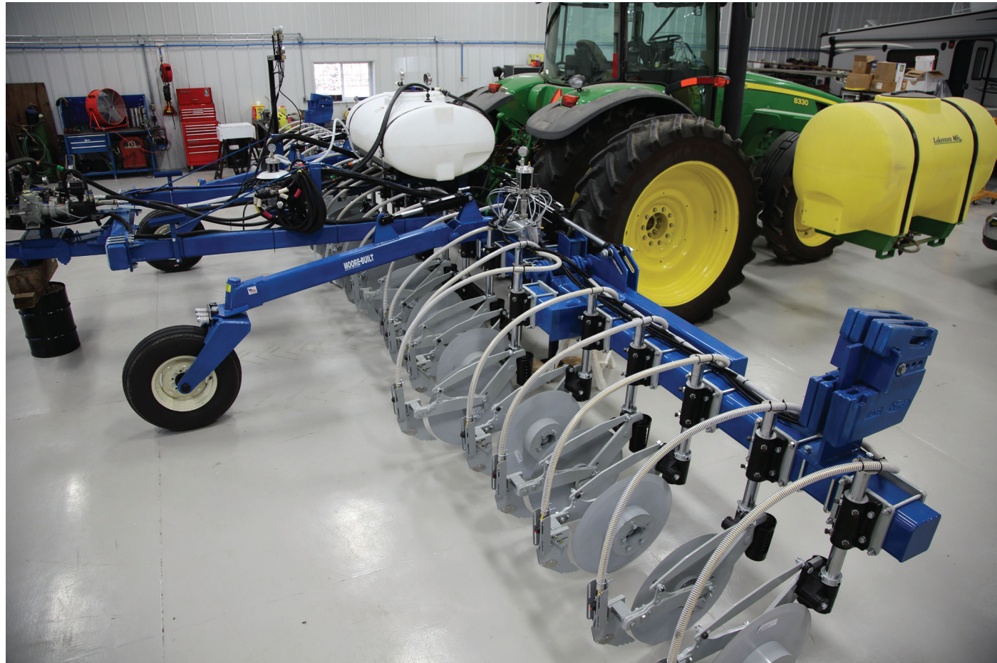
Mustang in 4 classes is another smart choice for producers requiring deeper bands at 7-to-8-inch depth. This is a top notch Mustang tool bar for raising corn yields in the 270-to-300 bushel-per-acre range, with 18-inch band centers in Twin Row Corn.
