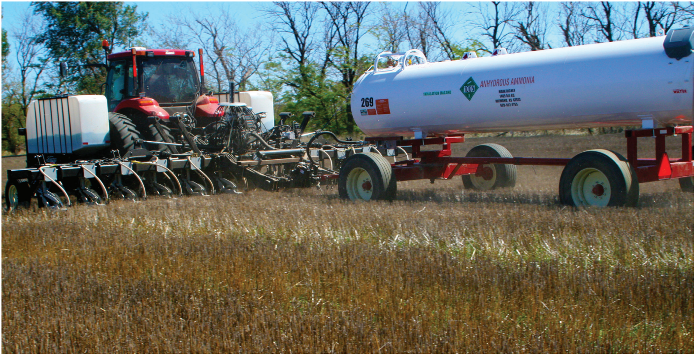
Demonstration of Mustangs in Lyons, Kansas, at 12.5 mph at a 7-inch depth; 30 feet at 15" band center, at .75 acres per minute.
