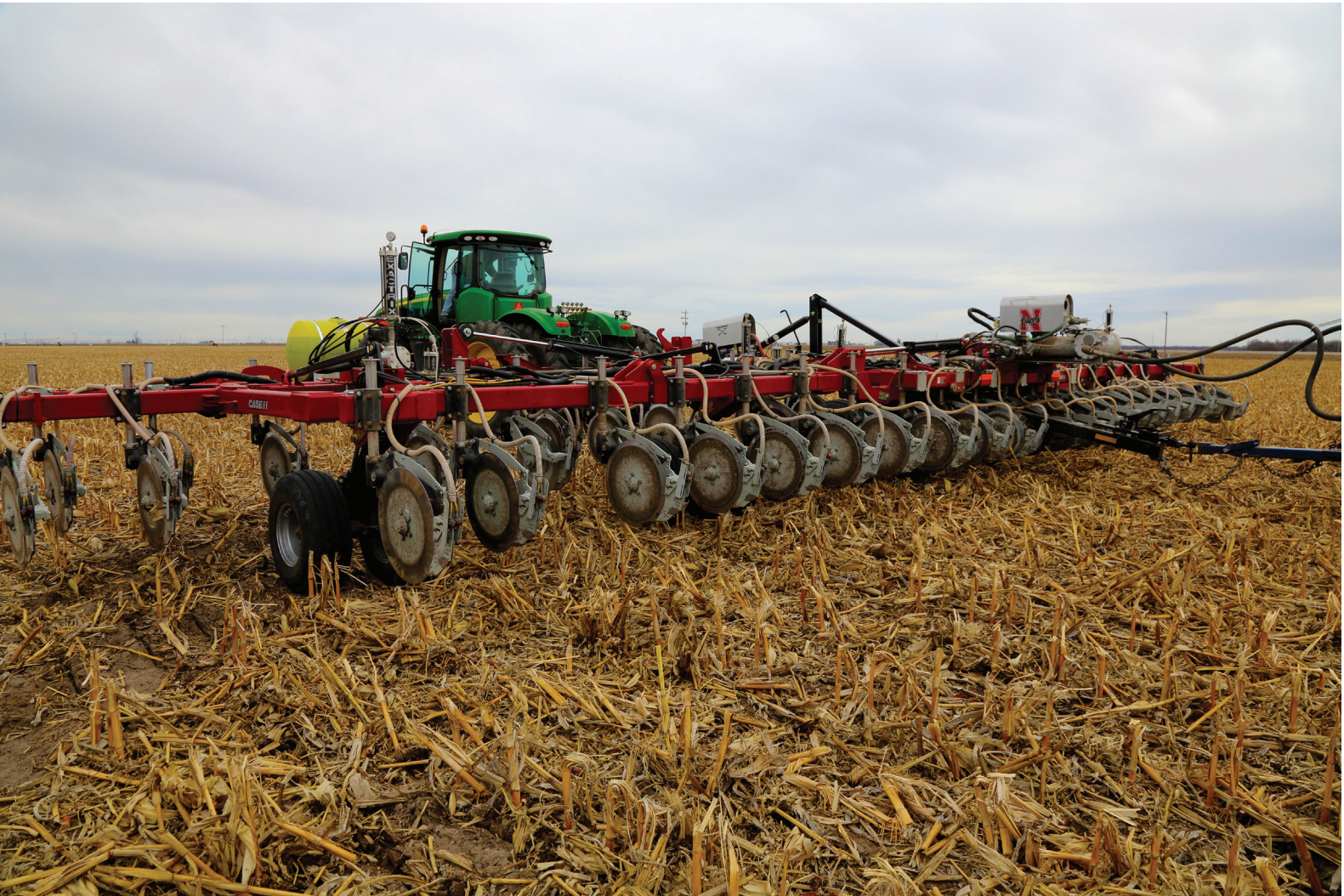
Case 940/Mustang at 61.5 feet banding No-till into irrigated 280 bushel corn stover, Shelton, NE
