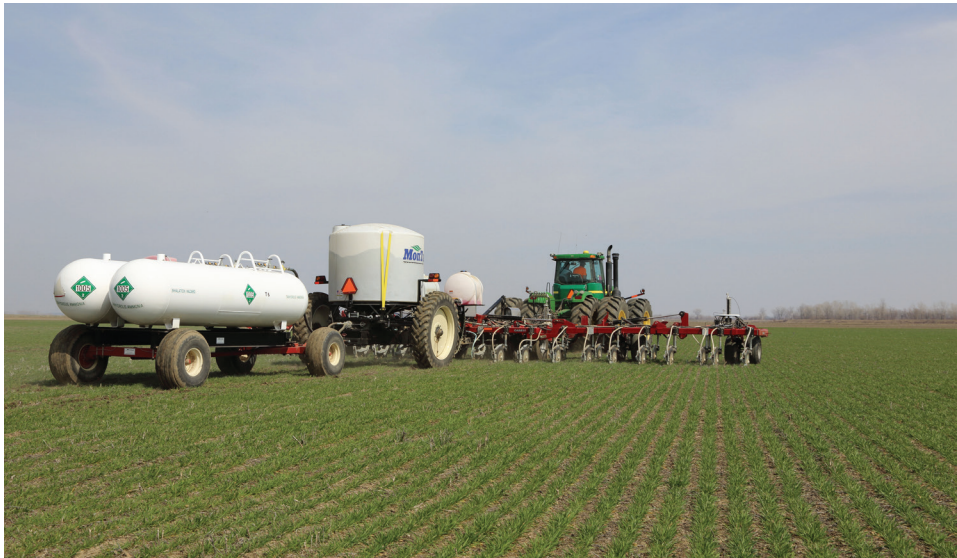
Case 940 banding in growing wheat. A five section machine at 50 feet with 15 inch band spacing.
