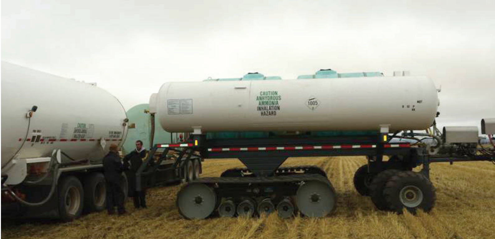
Dechant Farms has built 3 of their own design application trailers that carry 4,000 gallons of NH 3 and 2,600 gallons of liquid fertilizer. One trailer was recently sold to a large Nebraska farmer.
