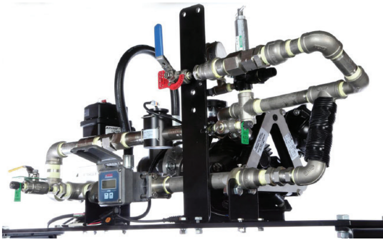
2KR Blenders assure accurate delivery of 3rd product for blending.
