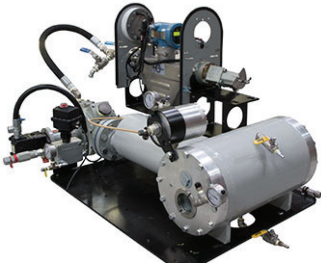
2KC, Series 3 NH3 system. Utilized on tool bars flowing between 20 to 40 gallons per minute NH3.
