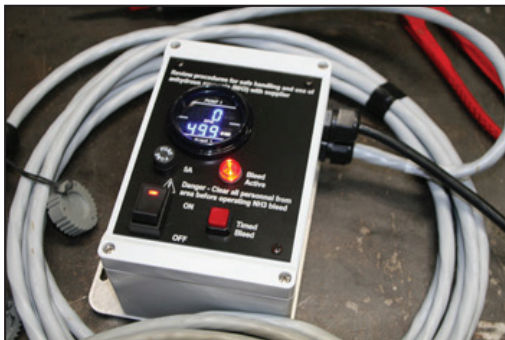
Timed bleed tachometers are for two systems. Series 2KC, 2KP, 2KR, 2KM
