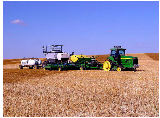
Small grains, Deere 1860, dual placement, 42.5 feet, 7.5 inch band spacing, 2KFA-NH3, Delta P-APP/S
