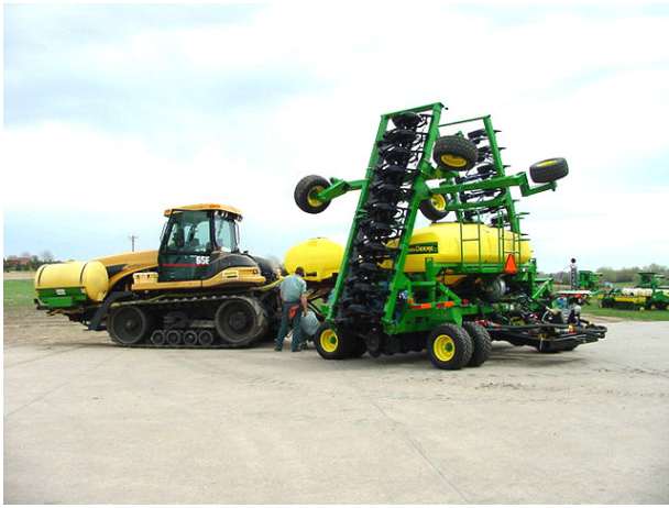
Corn Pre-Plant, Deere 1690 CCS, dual placement, 42.5 feet, 15 inch band spacing, 2KD Weigh Master-NH3, 2KM-APP/S
