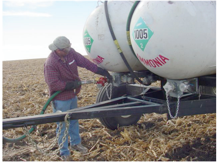
Easy and safe connections with remote bleeder lines and safety rope shutdown.
