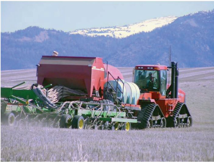
Lovell and Cook, Ririe, ID, 25 years continuous no till at 5,200 feet. Spring wheat seeding with a Deere 1895, AGPro seed metering, Yielder Drill and Exactrix.
