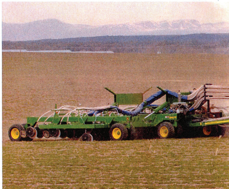
A CASE IH Quadtrac 535 pulls the one-pass wonder that fertilizes and drills wheat seed.
