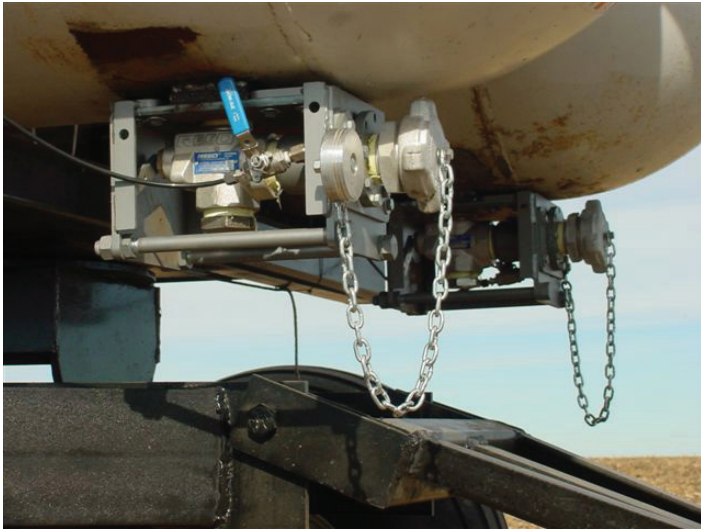
Exactrix 2 inch RT valves with guarding and parking caps. Approved in all states.
