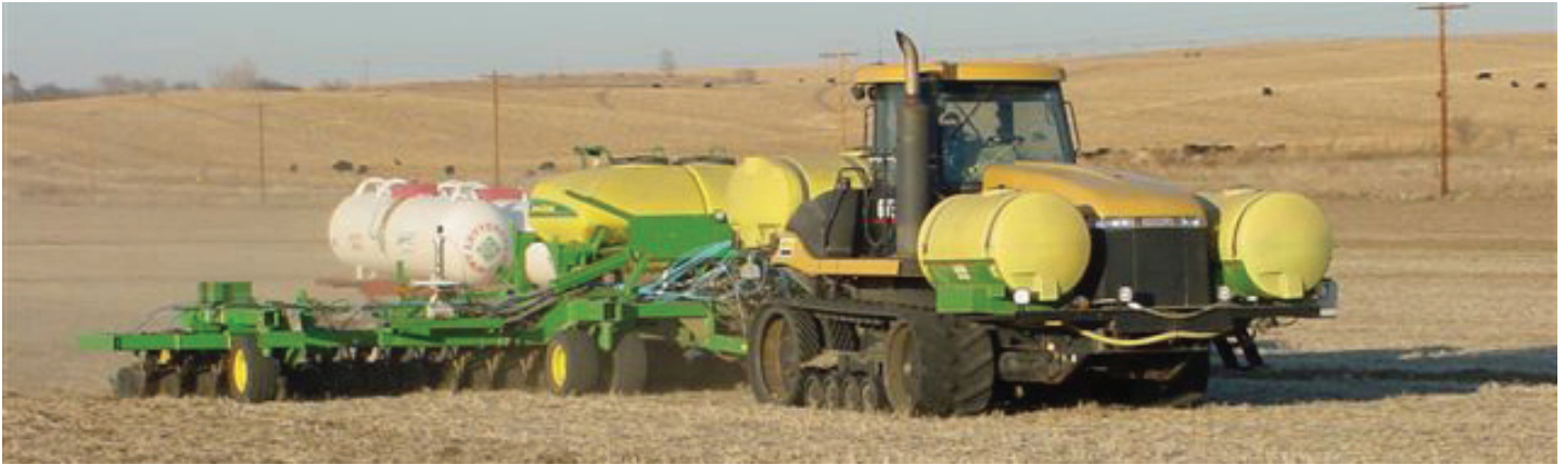
Albion, NE, a single pass winter wheat system or a two pass winter wheat system with the Deere 1690 CCS. A pre-plant nutrient tool for corn production. The first seeder to fertilize soy beans with wing injection of NH 3 , APP/APS.
