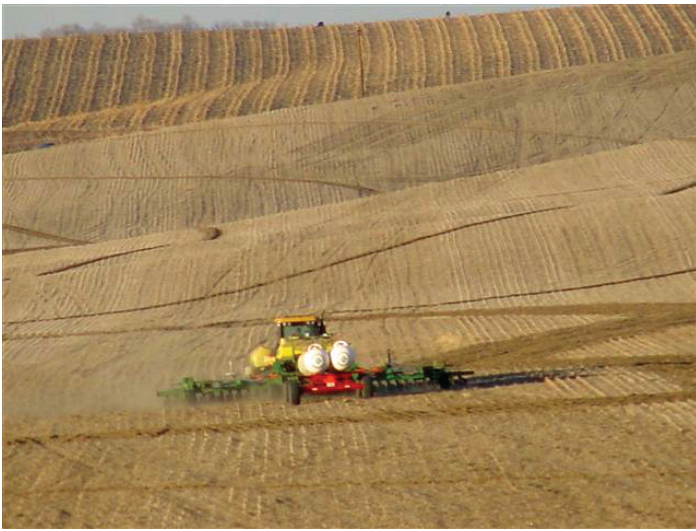
Deere 1890, 1990, an ideal pre-plant banding tool, 10, 12, 15 inch spacing.
