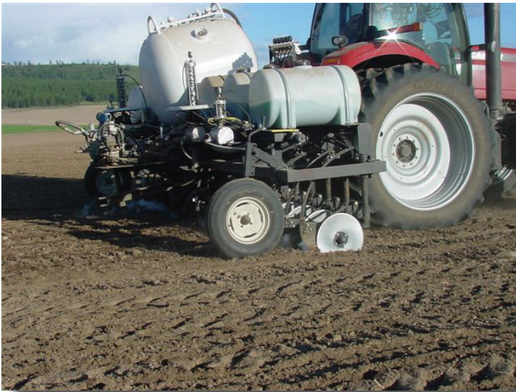
Single Disc Openers allow side dressing right after planting. Low disturbance P-51.
