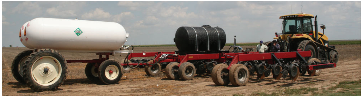
A two pass no-till applicator. Fertilizing winter wheat in side dress late fall application with a Case SDX 15 inch band center. The SDX has 32 openers and applies nutrients in the spring for irrigated corn production. Application speeds are 7 to 8 mph.
