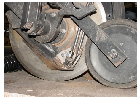
Deere 1890 wing injection will also fertilize soybeans. A powerful tool on the Great Plains.
