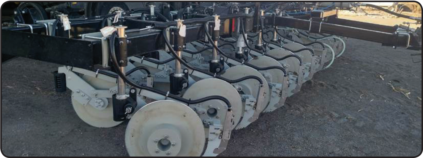
Mustang Banding for 30 inch winter Canola rows. The 30 foot bar has 15 inch band spacing., P-51C Mustang Openers.
